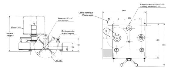
Height with standard set of weight: (bar, kPa): 445 mm (PSI): 420 mm Unit used: mm
