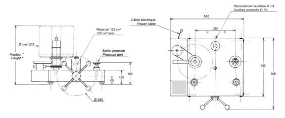
Height with standard set of weight: (bar, kPa): 420 mm (PSI): 385 mm Unit used: mm
