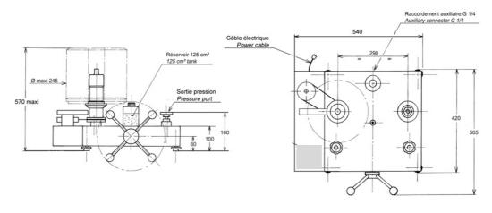
Height with standard set of weight: (bar, kPa): 375 mm (PSI): 370 mm Unit used: mm
