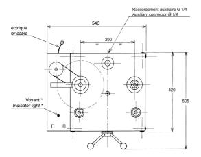
an automatic weight set motorization, which ensures regular rotation
