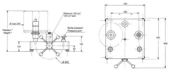
Height with standard set of weight: (bar, KPa): 500 mm (PSI): 490 mm
