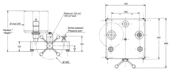
Height with standard set of weight: (bar, KPa): 445 mm (PSI): 420 mm
