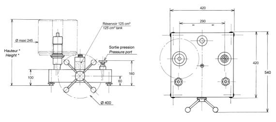
Height with standard set of weight : (bar) : 375 mm (PSI) : 370 mm
