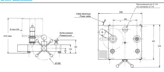
Height with standard set of weight: (bar, kPa): 411 mm (PSI): 386 mm
