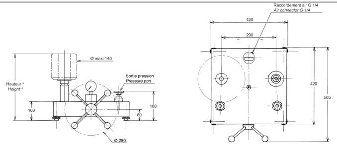
Height with standard set of weight : (mbar, mmH<sub>2</sub>O, kPa) : 315 mm
