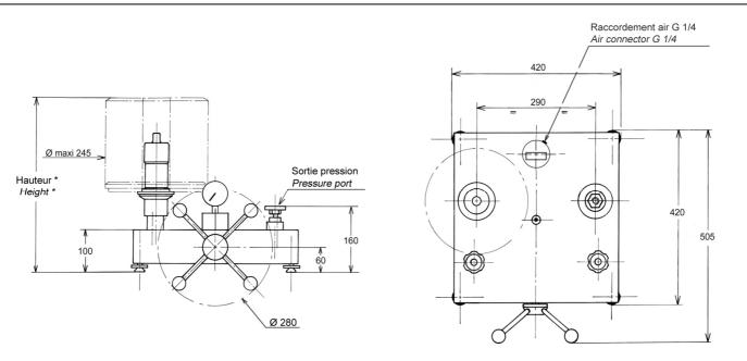
Height with standard set of weight : (bar, kPa) : 395 mm (PSI) : 379 mm
