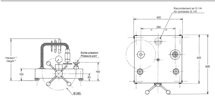
Height with standard set of weight : (mbar, mmH2O, kPa) : 410 mm
