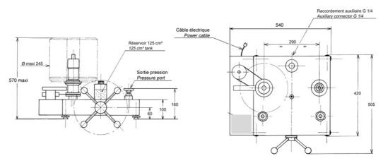
Height with standard set of weight: (bar, kPa): 375 mm (PSI): 370 mm Unit used: mm
