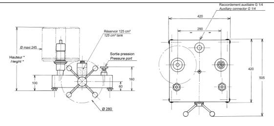
Height with standard set of weight : (bar) : 430 mm (PSI) : 420 mm
