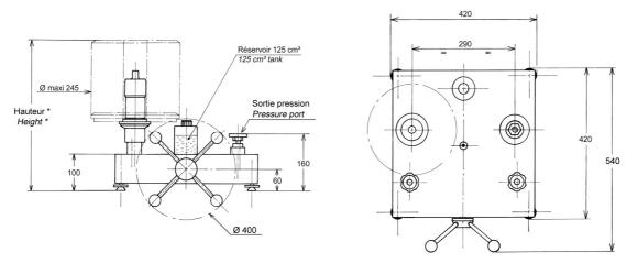
Height with standard set of weight: (bar, KPa): 500 mm (PSI): 490 mm
