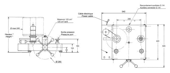
Height with standard set of weight: (bar, KPa): 450 mm (PSI): 465 mm Unit used: mm
