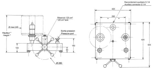
Height with standard set of weight : (bar) : 410 mm (PSI) : 420 mm
