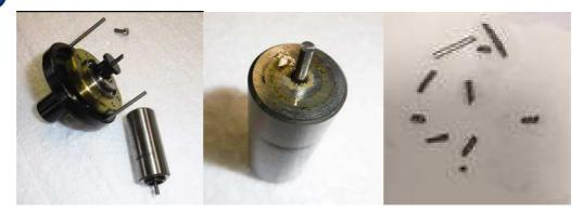
All our pistons are unique, because the last manufacturing step requires a honing operation carried out by hand by our technician. This operation is essential to obtain the best result of mobility and precision from your dead weight tester. It's therefore impossible for us to manufacture the same piston twice, each DWT is unique.
